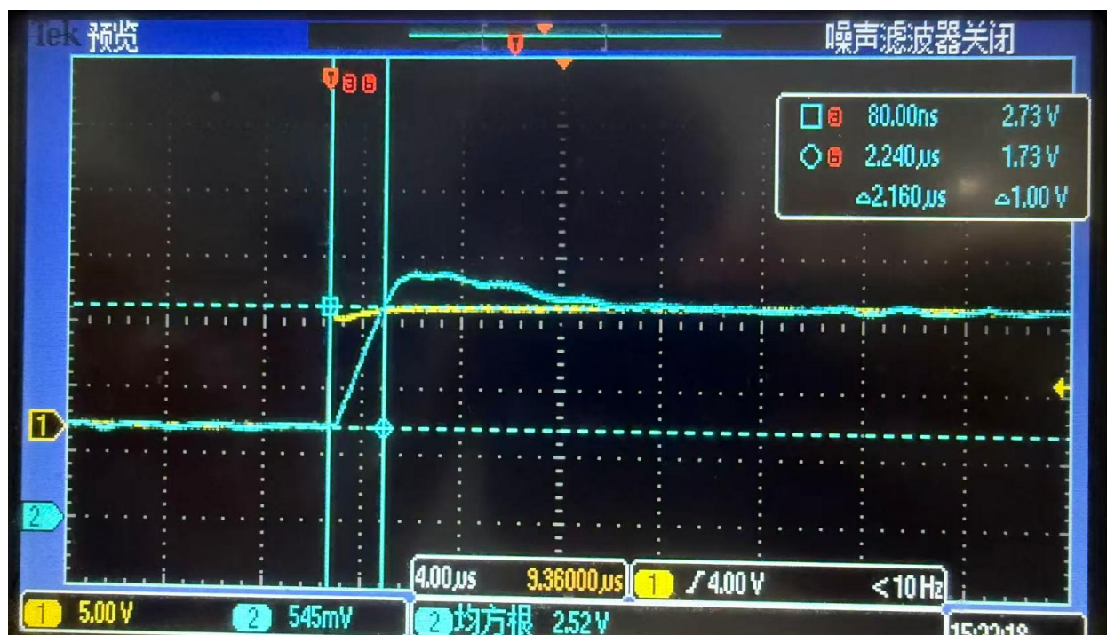
Fig.3 CH1 is primary magnetic field, and CH2 is output voltage; FFE-020F16T21SJR-020K series show output response time of 2.16 μs (~2 μs)
